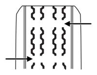
the same height as these "wear bars", the tire is worn out and must be replaced.
